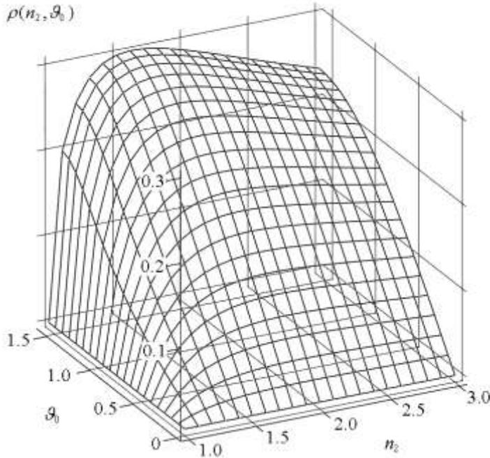
**Fig. 2.** Dependence of the effectiveness parameter of the transversal light dragging on refractive index  $n_2$  of the OD material and the incident angle  $\mathcal{G}_0$  (in radians).
