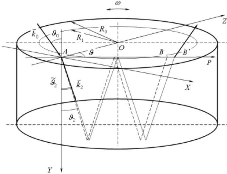
Let us an electromagnetic wave with a wave vector  $\vec{k}_0$  is incident onto a flat surface of a rotating with angle velocity  $\omega$  optical disk of a radius  $R_0$  under an angle  $\mathcal{G}_0$  in a plane  $YAP$  (fig.1).
