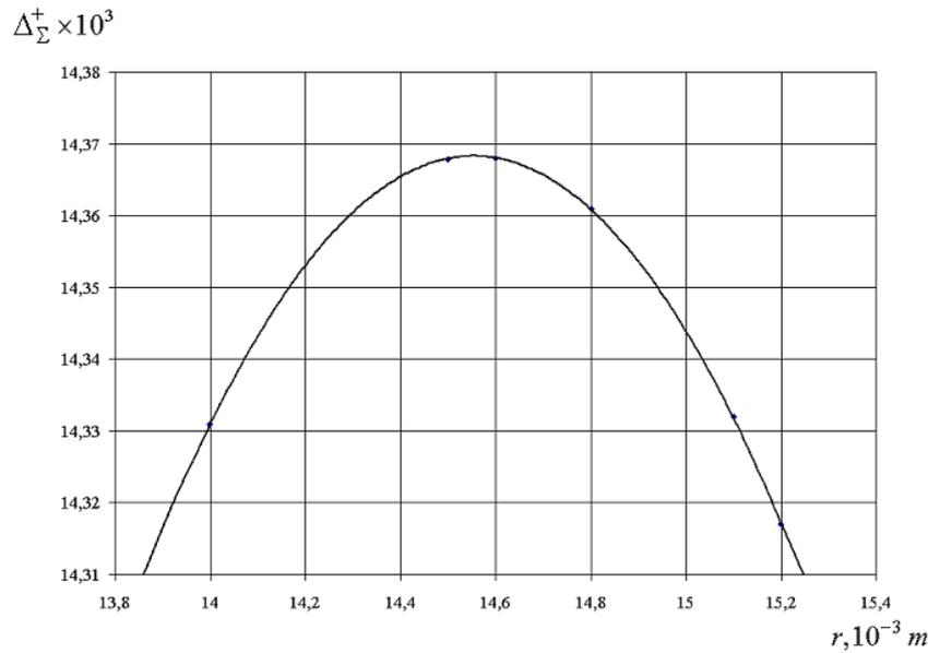
**Fig.3.** Dependence of the total optical path difference  $\Delta_{\Sigma}^+$  on the parameter  $r$ .
